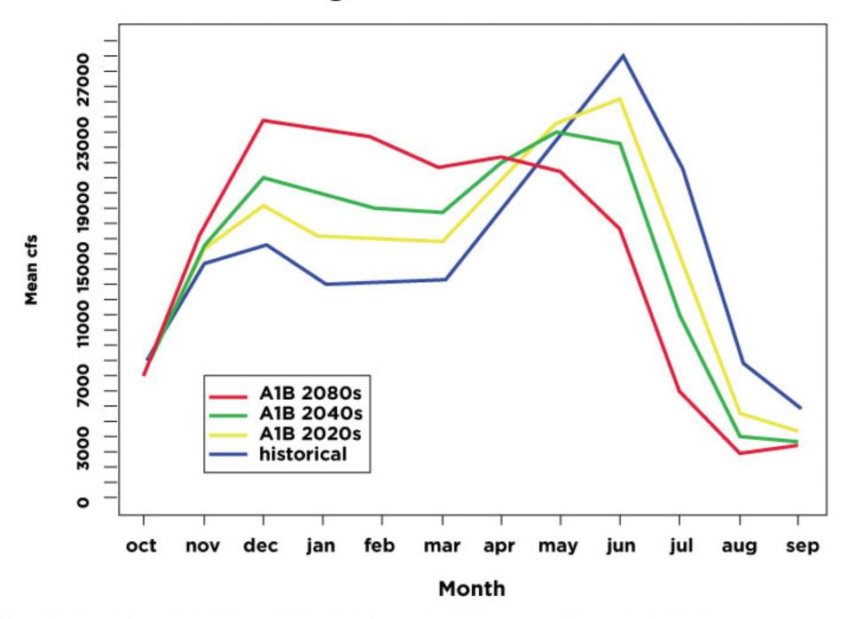
Hydrographs of projected monthly streamflows on the Skagit River at Mt. Vernon (starting in October). The lines represent simulations for the historical (blue), the 2020s (yellow), the 2040s (green) and the 2080s (red).
