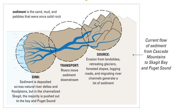
Some sand and gravel fills in river channels between dikes and levees, increasing the risk of flood (A). Dikes and levees steer sediment-laden waters away from valuable farmland and cities such as Mt. Vernon, Burlington, and Sedro-Woolley. Increased sediment puts pressure on levees as well as bridges during flood events.
